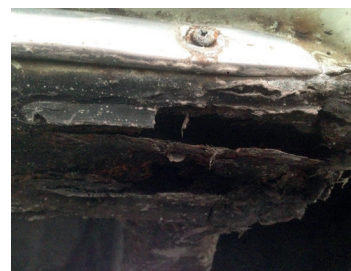
Corrosion to the sills required attention
