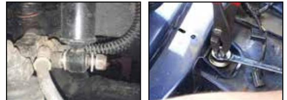
Figure 32-33, Component order as shown - hold shaft with Mole grips while the upper nut is tightened.
