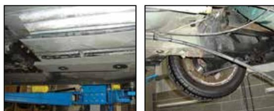
Figure 57-58, Lower hydragas pipes and gently pull through.
