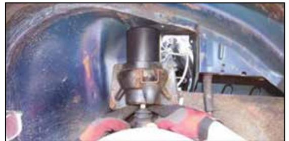
Figure 23, Lock the new unit in place.
