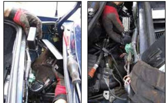
Figure 47-48, Disconnect the ECU connectors.
