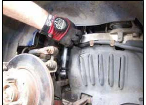
Figure 42, Fit the rear damper.
