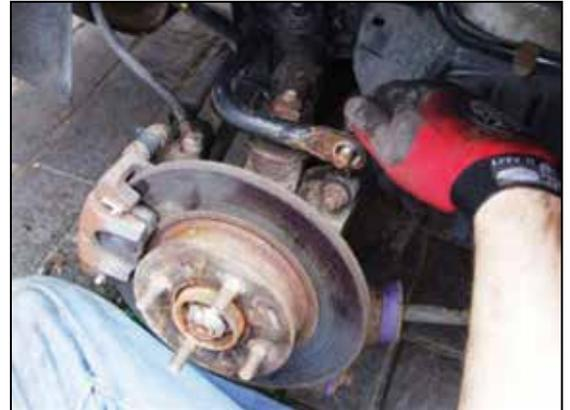
Figure 36, Undo and remove the anti roll bar to link top nut and bolt.
