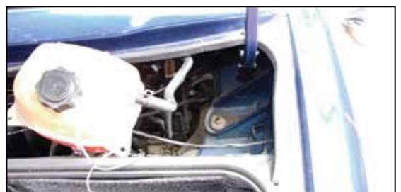
Figure 35, Move the coolant expansion tank.
