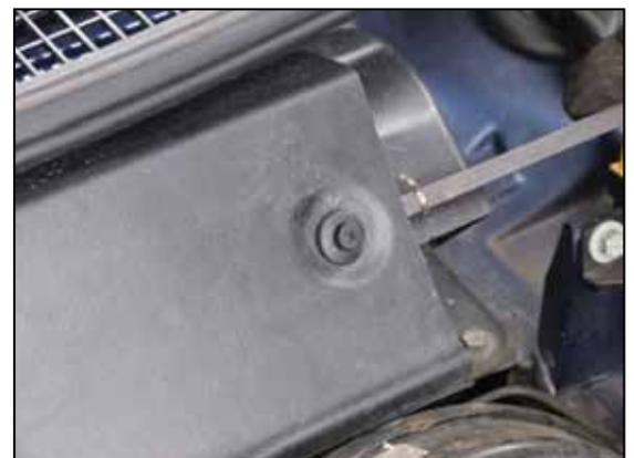
Figure 5, Prise out the rivet section.
