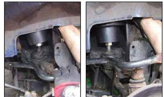
Figure 40-41, 'post' the new unit up between the body and subframe - before negotiating it into position.
