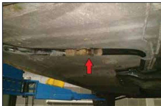
Figure 54, Chassis hydragas pipes.
