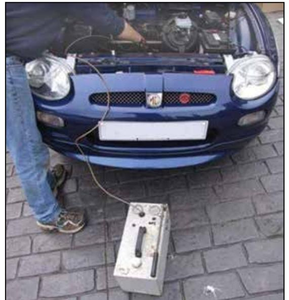
Figure 7, Hydrolastic pump and adaptor.
