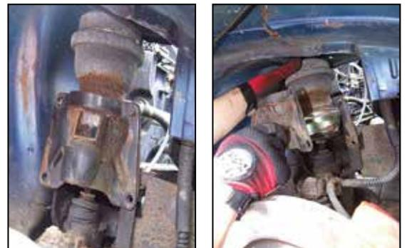
Figure 17-18, Remove the displacer.
