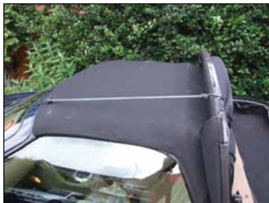
Figure 51, Hold spar in position.
