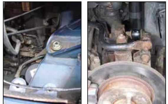
Figure 43-44, The upper nut torque is 50Nm - reconnect the rear anti roll bar, torque 45Nm.
