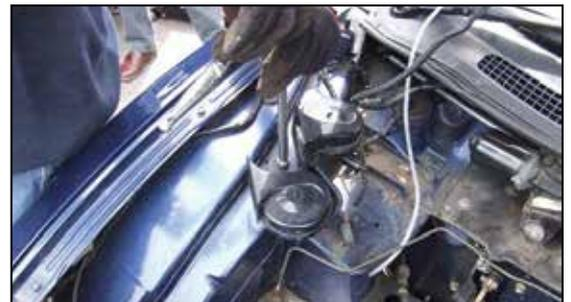
Figure 13, Remove horns and brackets.
