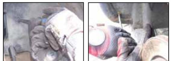
Figure 8-9, Undo scrivets and screws
