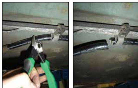
Figure 55-56, Cut hydragas pipes.
