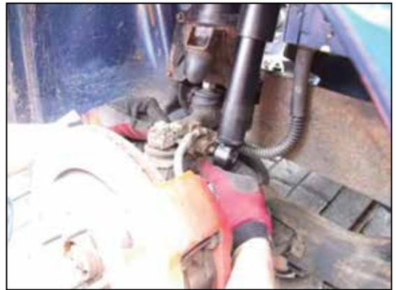
Figure 31, Refit the lower damper bolt.
