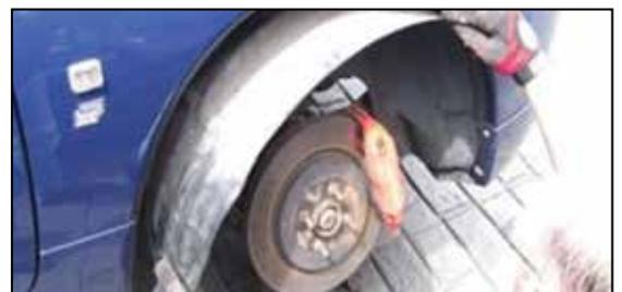
Figure 10, Peel out front inner wheel arch liner.
