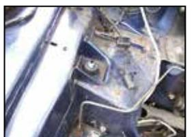
Figure 27-28, Feed threaded shaft through - replace rubber.
