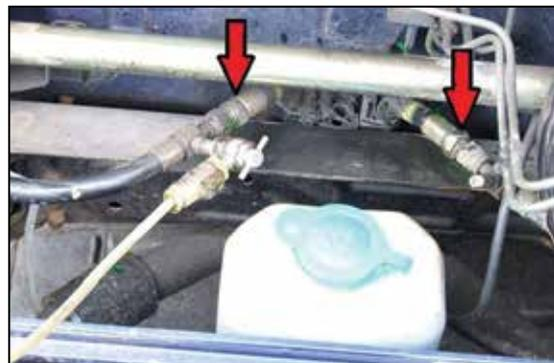
Figure 53, Disconnected hydragas pipes, front.
