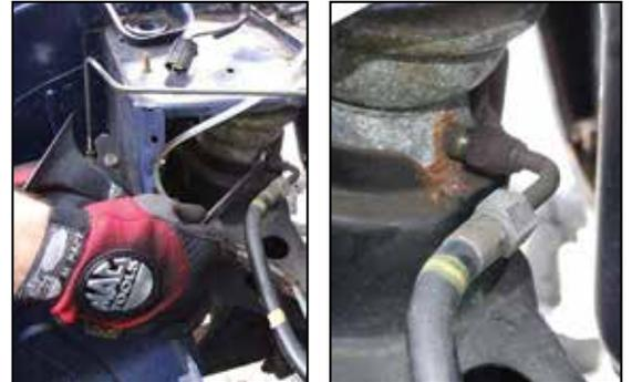
Figure 15-16, Remove pipe from displacer.
