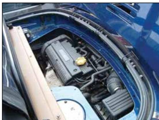
Figure 52, Remove engine cover.
