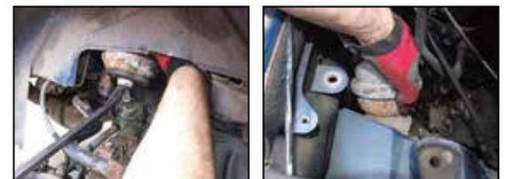
Figure 38-39, Lift out the displacer through the engine bay, rather than the wheel arch.
