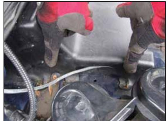
Figure 4, Undo the two 10mm plastic nuts.
