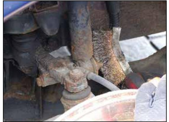
Figure 11, Wire brushing the nut and bolt.
