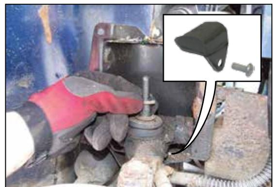
Figure 20, Retain the spacer washer.
