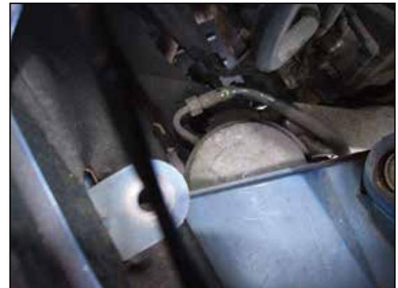
Figure 37, Remove the rear displacer.
