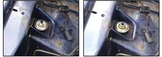
Figure 29-30, Replace concave washer (concave face, faces rubber) - and nyloc nut.
