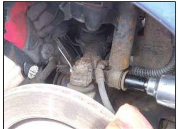
Figure 12, Note the correct positions of the brake hose clamp, spacer and two washers.
