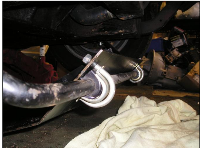
Fig 4: ARB centre mounts fitted to rally radiator shield.
