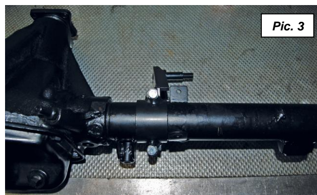
Pic 3. RH axle brackets in approximate position. Note: Fits between handbrake and brake hose brackets. File weld as required to allow good fit.
