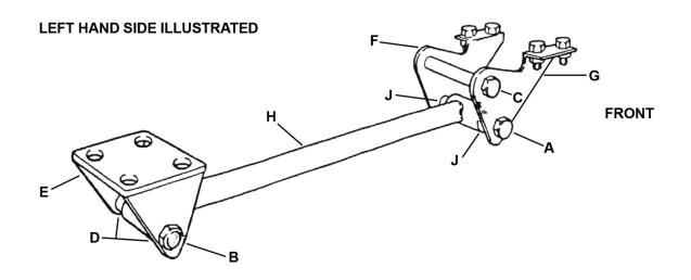
3. Jack up the car and support on axle stands just forward of the front eye bolt mounting for the leaf spring, this then allows the axle to swing free.
