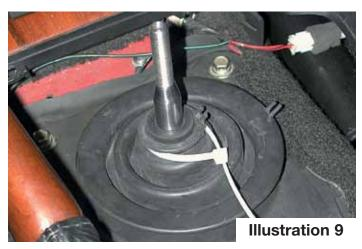
10. Re-install the sound deadening material and the center console. Take care to pass the Fuel door/Trunk levers through the rear of the console first and then re-fasten with the mounting screws. Complete the installation by re-installing the shift knob.
