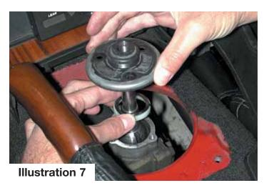
8. From the kit, slide the black rubber bushing down the shaft of the lever until it stops against the shoulder above the inner boot.
