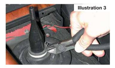
Remove the dust boot to expose the shift lever and the top of the transmission.
