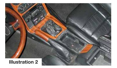
Gently lift the console at the front and pull it forward to release the fuel door/trunk lever(s) from the rear of it. The console will not pull completely free of the car, as it will have some wires attached to the bottom of it. Gently lay the console across the passenger's seat so that you can gain access to the shift lever.
