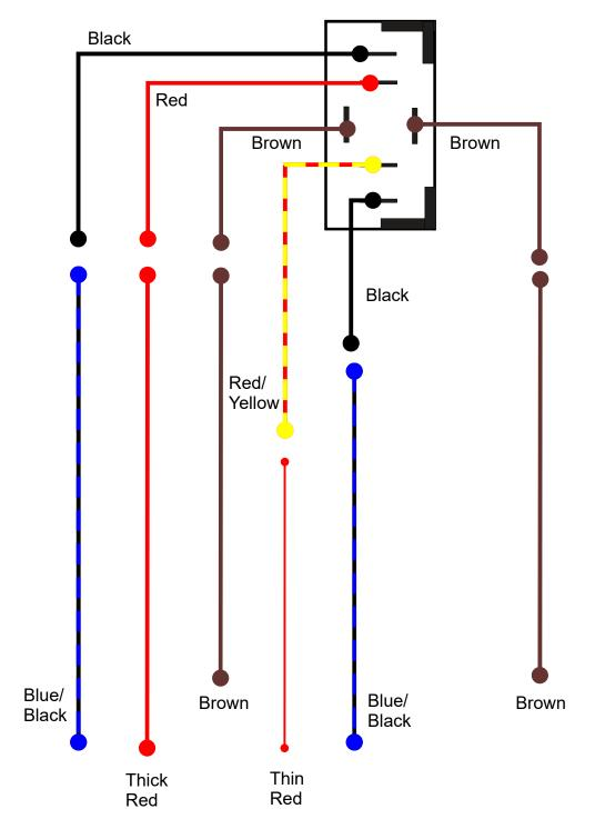
Blue/Black wires run to electric window motors.
