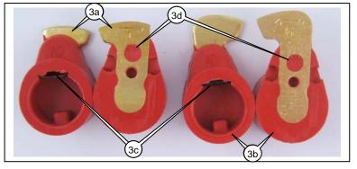
This "miss" will sometimes heal itself if the engine is given a chance to cool off, but it always comes back, and in the end, the rotor will simply short out completely, which could leave you stuck on the side of the road.
