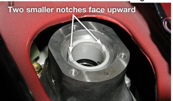
21. Install the lockout plate on top of the spacer adapter. Locate the three provided hex-head bolts. Drop a bolt into each of the three holes in the top of the shifter. Tighten each bolt to 7.5 ft. lbs. or 90 in. lbs. Figure 21.
