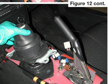
13. Pull up around the circumference of the lower shift boot to dislodge it from the transmission tunnel. Then pull it off of the shifter. Figure 13.
