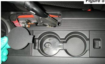
6) Remove the screw under the front cupholder. Figure 6.
