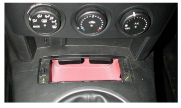
4) Remove two phillips-headed screws under the change holder. Figure 4.
