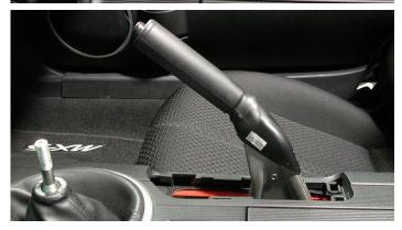
3) Use a screwdriver to remove the plastic change holder. Figure 3.
