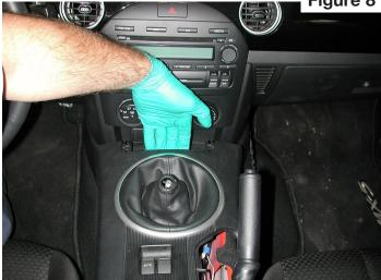
9) Lift the center console 6 to 8 inches and slide a hand underneath. Disconnect the power window switch harness connector. Squeeze the tab to release the connector. Figure 9.
