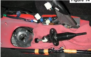
15. Turn the black shifter ball bushing slightly so that there is a gap between the metal of the shifter and the bushing. Stick the flat blade of the screwdriver through the hole in the bottom of the shifter cup. Use the flat edge to pop the black plastic shifter ball bushing off of the shifter ball. It should come off relatively easily. If it does not, move the black shifter ball bushing slightly and try again. Figure 15.
