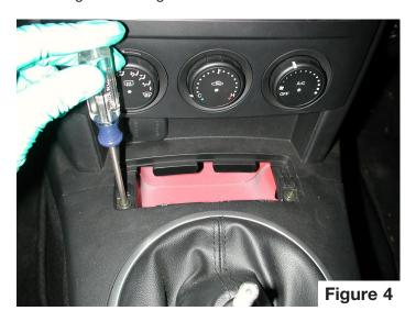
Slide the cupholder cover back. Remove the floor of the first cupholder. Figure 5.
