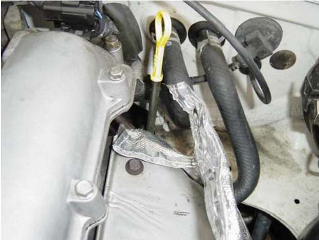
Photo 2-A: Right side of the Heat Shield. Fold in first followed by the top
