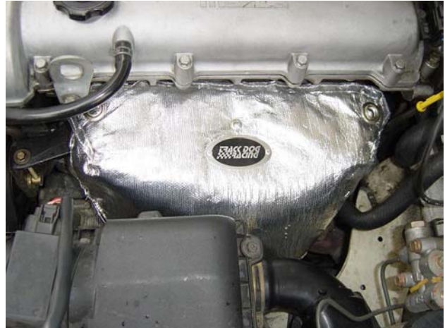
Photo 2-B: The center hole is between the two valve cover bolts and a rib on the head
