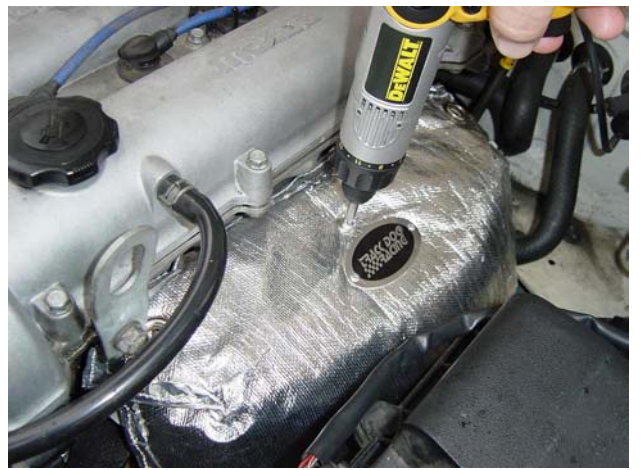
Photo 2-F: Form the Heat Shield back around the factory manifold and attach the self-tapping screw
