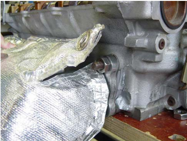
Photo 1-A: Right side of the Heat Shield. Fold in first, followed by the top
