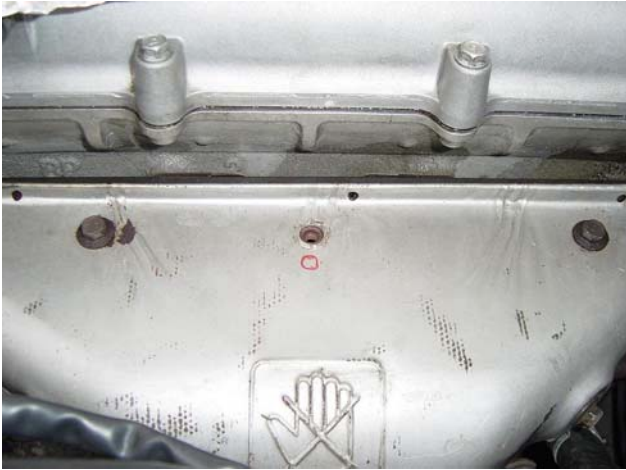
Photo 2-C: Mark the hole on the header shield centered with the head rib between the two valve cover bolts
