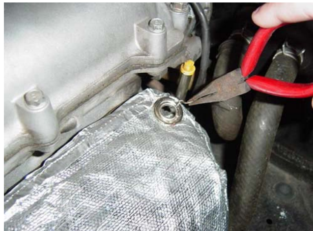
Photo 1-F: Stainless steel wire on right side of factory manifold with shield removed
