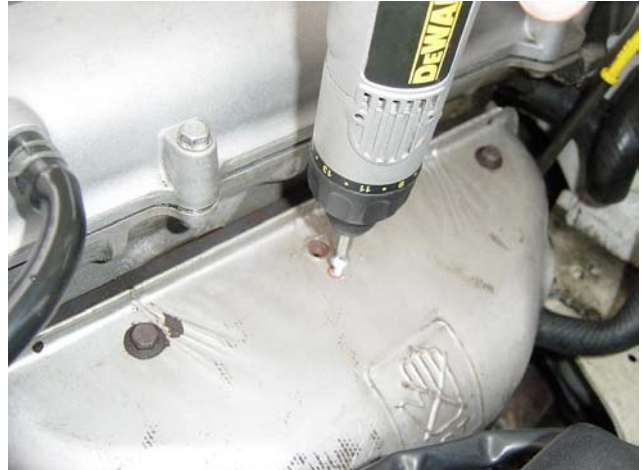
Photo 2-D: Screw the self-tapping screw into the factory metal shield, then remove for reinstall
