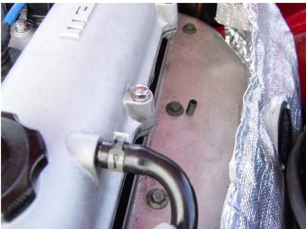
Photo 2-E: Spacer between the Heat Shield and the factory exhaust manifold
