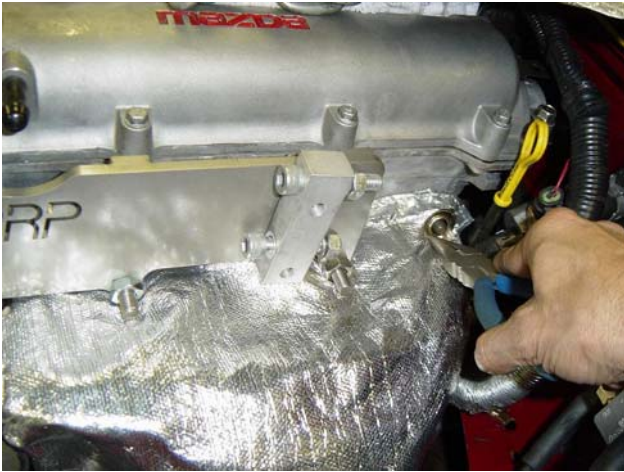
Photo 1-C: Using a tool to push the grommet around the stud
