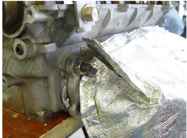
Photo 1-B: Left side of the Heat Shield. Fold in first, followed by the top
