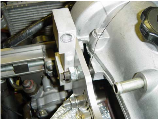
Photo 1-E: Stainless steel wire on left side behind supercharger bracket
