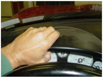
Photo 3-D: Pull the bezel top to release from the spring-clips
