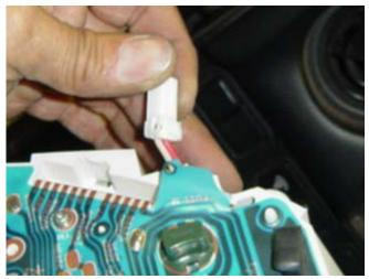
Photo 2-G: See note above on removing the 2-wire connector
