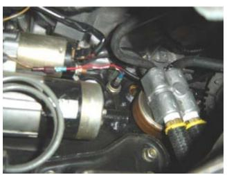
Photo 1-B: Location of the stock oil pressure sender
