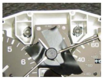
Photo 4-B: Using two small screwdrivers, apply even pressure to release the pointer
