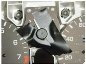
Photo 4-A: Use electrical tape on the face of the gauge panel to protect it
