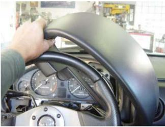
Photo 2-E: Lay dashboard bezel off to the side
