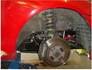
Photo 1-A: Remove the tire for access through the fender well
