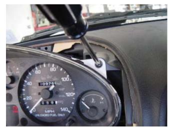
Photo 2-F: Remove the 4 Phillips screws that attach the gauge panel to the dashboard
