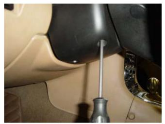
Photo 3-A: Remove the steering column cover
