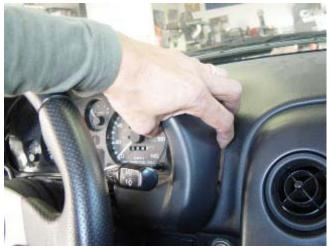
Photo 2-D: Grip the dashboard bezel and pull to release the spring-clips
