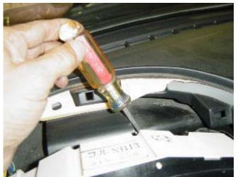
Photo 2-H: Remove the speedometer cable by using a screwdriver to press the release clip
