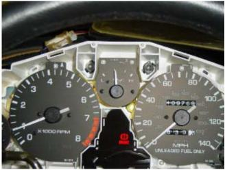
Photo 4-D: Oil pressure pointer at idle
