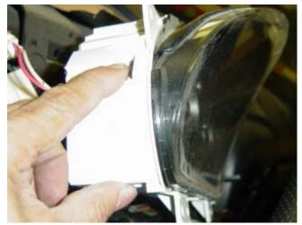
Photo 2-I: Remove the front cover by pressing the release clips around the perimeter
