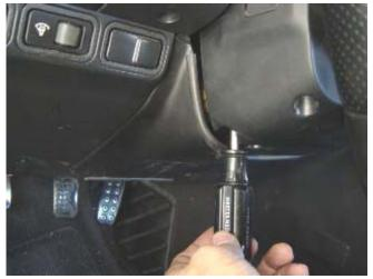
Photo 2-A: Remove the screws holding the steering column cover on with a Phillips screwdriver
