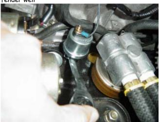
Photo 1-C: Use a 1/2" open-end wrench to tighten the new oil pressure sender
