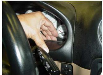
Photo 3-B: Remove the bezel by pulling to release
