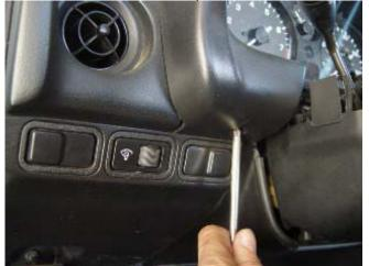
Photo 2-C: Remove Phillips screw in the dashboard bezel
