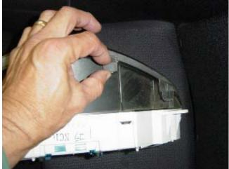
Photo 3-F: Remove clear cover by pressing on clips
