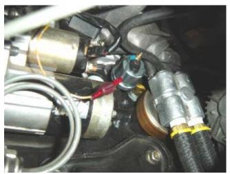
Photo 1-D: Attach the sensor wire to the oil pressure sender
