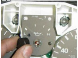
Photo 4-C: Pointer removed from the gauge
