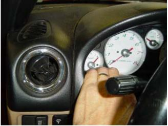
Photo 3-C: Using your fingers, reach between the bezel and the gauge panel and pull to release
