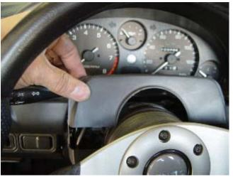
Photo 2-B: Remove the top half of the steering column
