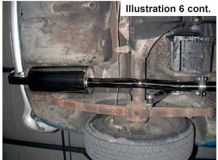
6. Gather the remaining hardware and gasket. Slip a flat washer onto each bolt. Apply lubricant to the upper hole in the rubber hanger on the rear of the muffler. Install the tail pipe (muffler) in the car by sliding the rubber hanger over the hook at the rear of the car. Align the flanges, slip a gasket in between, then install a bolt, flat washer, lock washer, and nut into each hole. Align the connection and tighten the bolts.
