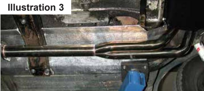
4. Next, slip the rubber hangers onto the hooks on the rear of the mid-pipe and the rear of the muffler. Use the longest hole in the rubber hanger. Apply silicone lubricant (or WD-40) to make installation easier.
