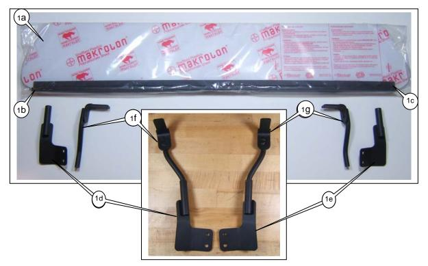
The two lower brackets (1d, 1e) are secured to the tapped plates that anchor the top frame just behind the door opening. The upper brackets (1f, 1g) have flat "tabs" that slide into the open ends (1b, 1c) of the rail that supports the windblocker (1a).
