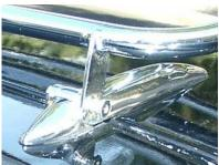
The support struts are secured to the lower lip of the trunk lid and were designed to rest on top of the bumper face bar. This was a poor idea, and Ron Phillips came up with a nifty idea- positively locate the ends and bring them in to sit on top of the bumper irons.
