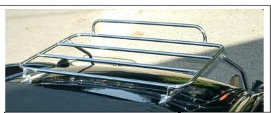
Rack is secured to the OE trunk hinges, which have hinge pins that can be pressed out. The hinges Moss sells are not useable because the chrome plating is done after the pin in inserted. If you push the pin out, you will chip the chrome.
