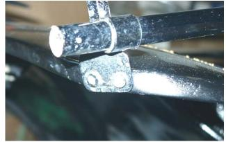
The support struts is hollow. It fits over the top of a pin which is secured inside the "V" in the bumper irons by cotter pins. The support strut actually is resting on the cotter pin.
