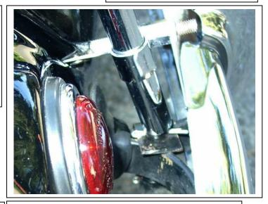
The support struts are secured to the lower lip of the trunk lid with screws and I suggest Nyloc nuts. Some people use pop rivets but those will work loose over time. You will have to work the location of the brackets out based on trial fitting the pieces.
