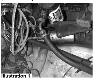
Remove the coil and it's primary bracket from the mounting bracket using a 7/16" wrench and socket tools. Locate a new place for the coil as shown, using the primary bracket to mark the hole locations. (Illustration 2) Using a center punch and hammer, make two dimples at the center of the marks. This will insure that the drill bit will not walk around when the holes are being started. (Illustration 3)
