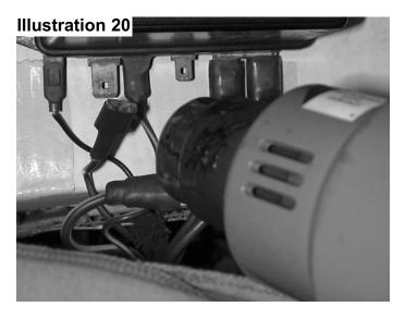
Attach the Brown/Green wire to the "D" and mount the regulator. If the regulator is utilizes screw type post then follow the same procedure omitting the modifications to the wires.
