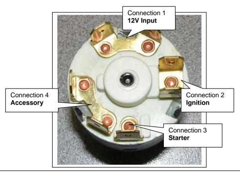
This switch has 3 positions and was originally supplied for Triumph applications. It is a good replacement for the original MG two position switch as it incorporates an Accessory position which is really useful for feeding a stereo and or 12 volt auxiliary outlet.
