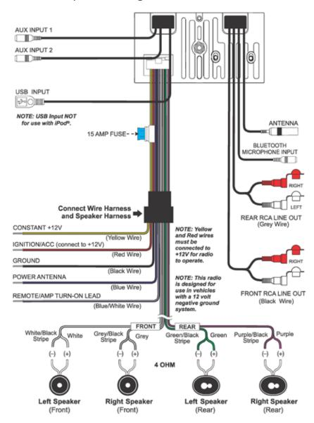
Figure 5 - Wiring Diagram
