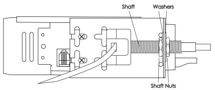
Figure 3 - Mount Shafts to Brackets
