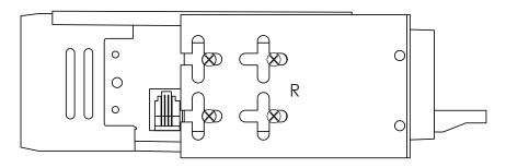
Figure 2 - Attach InfiniMount Brackets
