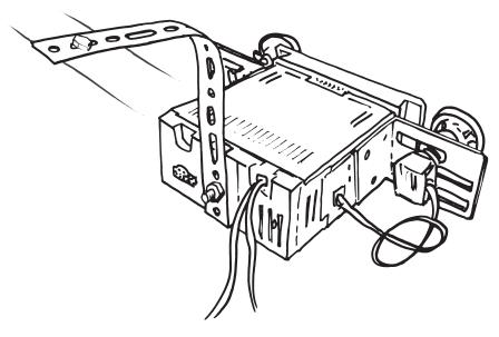
Figure 6 - Installing the Back strap
