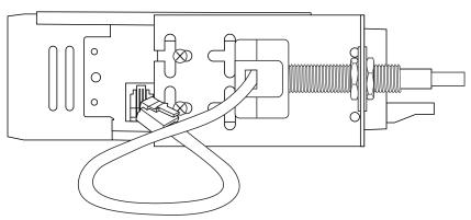
Figure 4 - Plug Shafts into the Body
