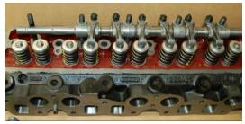
**3.5** Install the original washer; install rocker No.3, then spacer, then rocker No.2. Install rocker No.1 with Thackeray washer into No.1 pedestal and fit to the shaft.
