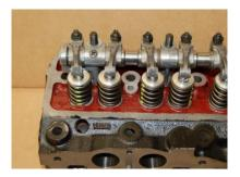
3.8 When you are satisfied with the set up, fit the split pin to the front end of the rocker pedestal No.1.
