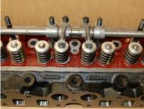
**3.3** – Install rocker No.5, new spacer and rocker No.4. There are no original washers used here. Then fit pedestal No.2.
