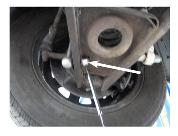
3. Using a 1/2in socket, short extension and a ratchet, remove the four four bolts that secure the factory anti-sway bar brackets to the vehicle. Then remove the factory anti-sway bar from the vehicle by lifting it upward while turning it towards the front of the vehicle, allowing the factory sway bar links to clear the steering arms as the bar is removed.
