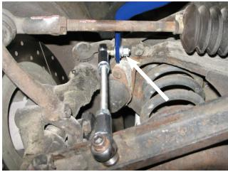
13. Use a 1/2in combination wrench on the upper anti-sway bar link stud and a 9/16" combination wrench on the nut to tighten the upper anti-sway bar link stud to **22 ft-lbs**. You'll want to be sure the lockwasher is fully compressed but not strip the threads of the upper link stud.
