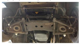
2. Using a 3/4in combination wrench, remove the nuts attaching the bottom of the front anti-sway bar end links to the a-arms. Then pull the stud of the end links out of the holes in the a-arms. You may need to wiggle the sway bar end link while tapping the lower stud of the sway bar link in order to free the lower sway bar link studs from their holes in the a-arms.
