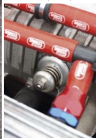
Over-pressure relief valve dumps excess boost if Oz closes the throttle rapidly. It doesn't get used much
