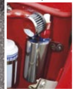
Crankcase vents lead to catch tank to stop oil mist feeding into the combustion cycle
