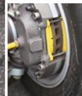
Big power needs big brakes. KAD four-potters can almost make this Mini stand on its snout
